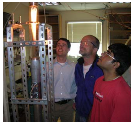
Dr. Moosmüller and graduate research students working on an inverted methane diffusion flame for the generation of black carbon aerosols
